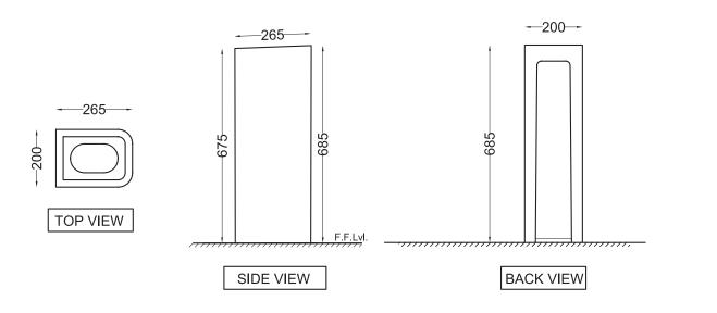
ALL DIMENSIONS ARE IN MM. (TOLERANCE ± 5 MM)
