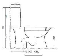
SIDE VIEW ALL DIMENSIONS ARE IN MM. (TOLERANCE ± 5 MM)
